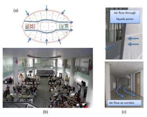
Figure 5. (a) Air flows through façade pores. (b) Cross ventilation system at Canteen area. (c) Air flow at coridor.
